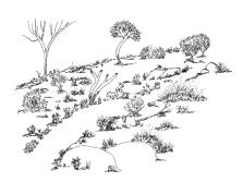
When making walkways and roads, plan to build them on land with a gentle slope. If the slope is steep, then build the walkway or road along the side of the slope gradually increasing in height. If the walkway or road is built straight up the slope, the storm water from the rain will quickly wash it away making it unusable. When planning walkways and roads, look at the slope of the land first, then it will be easy to see where to build them.
